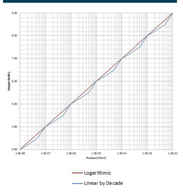
Analog output scaling example, see the specific controller/active gauge manual for all available analog output scaling options.
