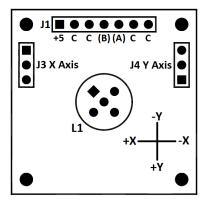
Note that the direction of measurement only applies when a dual axis sensor is mounted on the PCB.
